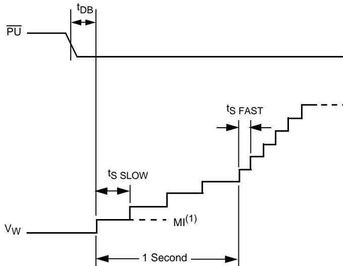
**Note:** (1) MI in the A.C. timing diagram refers to the minimum incremental change in the wiper voltage.
