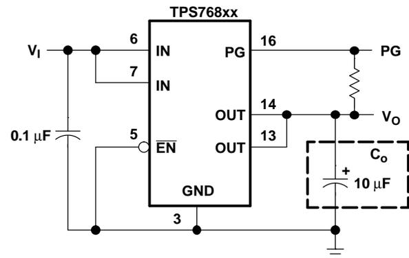
**Figure 1. Typical Application Configuration (For Fixed Output Options)**
