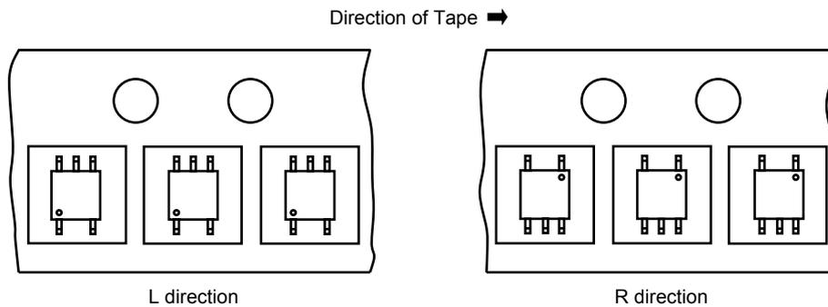
**Figure 1 Device Orientation**
