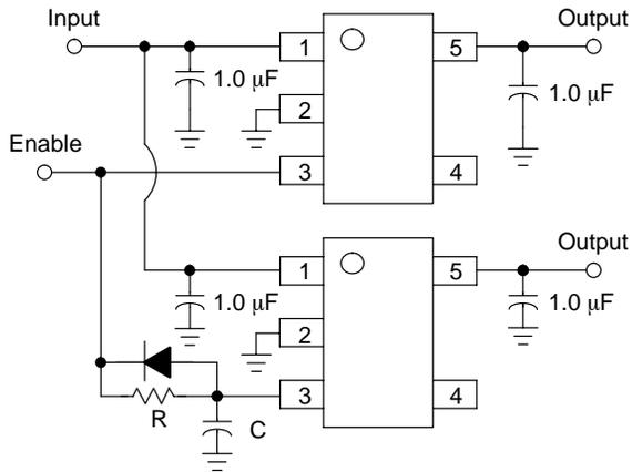
**Figure 23. Delayed Turn-on**
