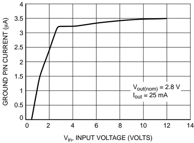
**Figure 4. Ground Pin Current versus Input Voltage**
