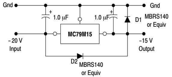
**Figure 2. Protection Diodes**
