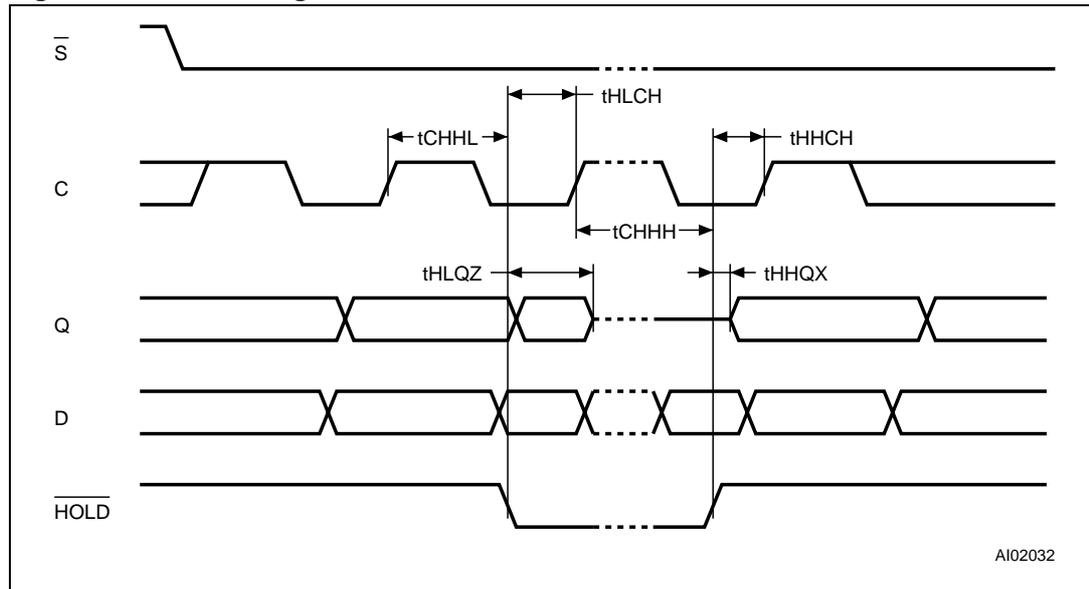
Figure 24. Output timing
