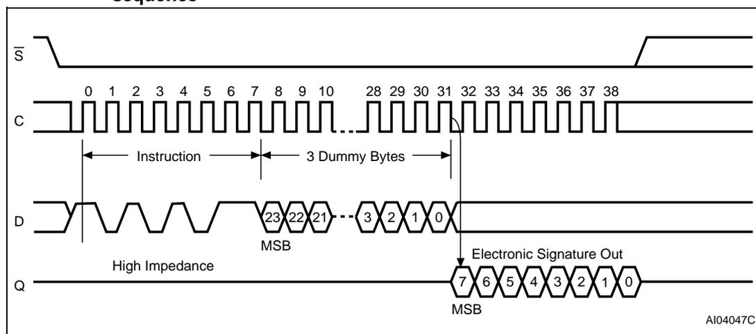
1. The value of the 8-bit Electronic Signature, for the M25P64, is 16h.
