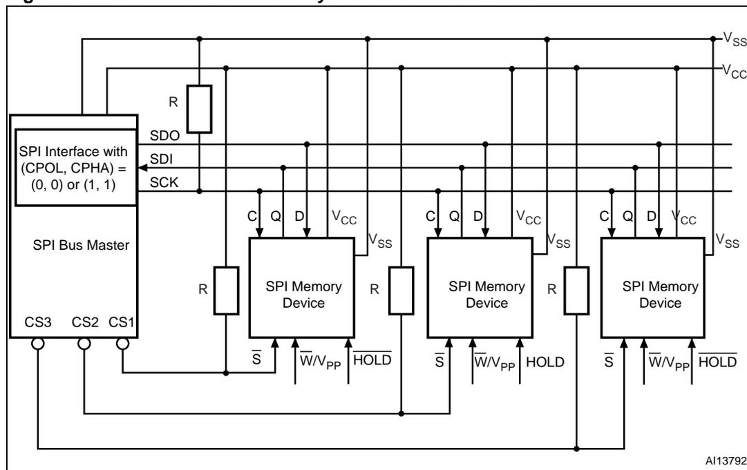
1. The Write Protect ( $\overline{W/V_{PP}}$ ) and Hold ( $\overline{HOLD}$ ) signals should be driven, High or Low as appropriate.
