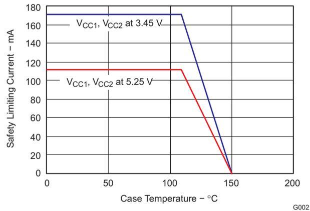
Figure 5.  $\theta_{JC}$  Thermal Derating Curve per IEC 60747-5-2
