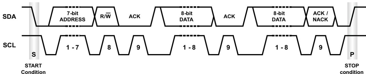
Figure 7. Timing Diagram of a Complete Data Transfer
