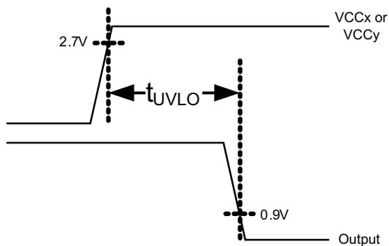
Figure 4.  $t_{UVLO}$  Test Circuit and Timing Diagrams
