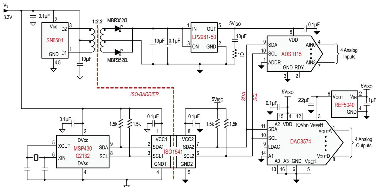
Figure 11. Isolated I<sup>2</sup>C Data Acquisition System
