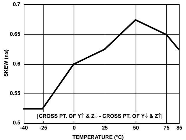
FIGURE 17. DRIVER DIFFERENTIAL SKEW vs TEMPERATURE (ISL83086E, ISL83088E)
