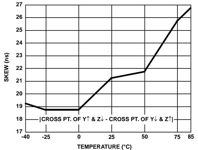
FIGURE 15. DRIVER DIFFERENTIAL SKEW vs TEMPERATURE (ISL83083E, ISL83085E)
