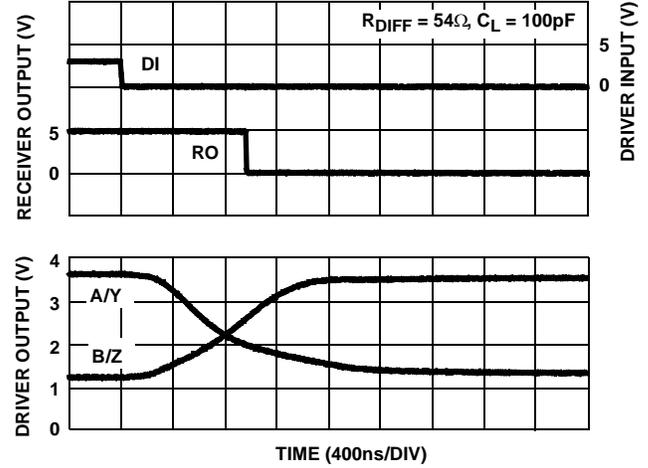
FIGURE 19. DRIVER AND RECEIVER WAVEFORMS, HIGH TO LOW (ISL83080E, ISL83082E)
