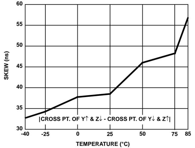
FIGURE 13. DRIVER DIFFERENTIAL SKEW vs TEMPERATURE (ISL83080E, ISL83082E)
