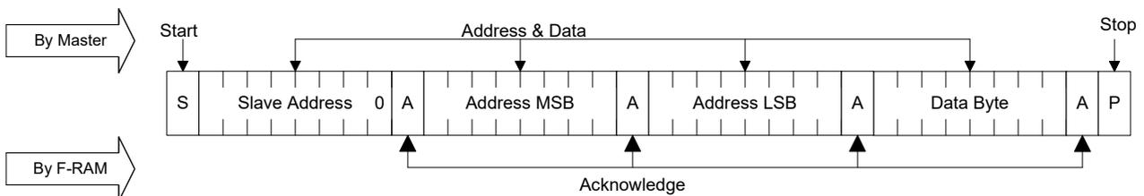
Figure 8. Multi-Byte Write
