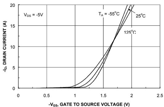
**Figure 5. Transfer Characteristics.**
