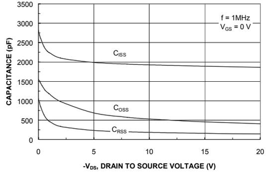
**Figure 8. Capacitance Characteristics.**
