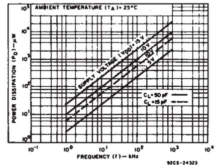
Fig. 3 – Typical power dissipation vs. frequency.
