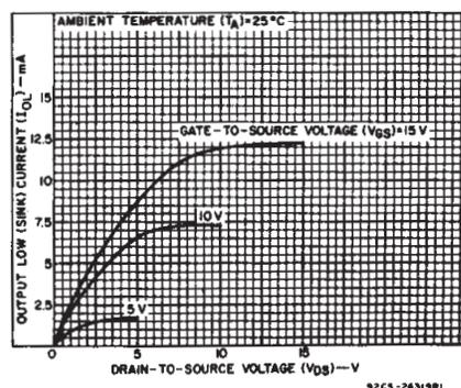
Fig. 8 - Minimum output low (sink) current characteristics.
