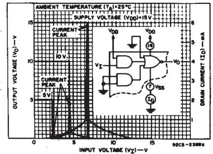
Fig. 1 – Typical voltage and current transfer characteristics.
