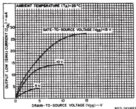
Fig. 7 - Typical output low (sink) current characteristics.
