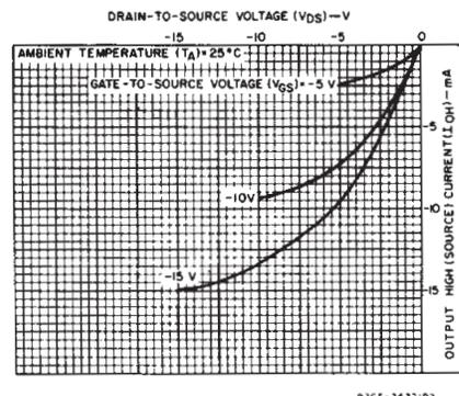
Fig. 11 - Minimum output high (source) current characteristics.
