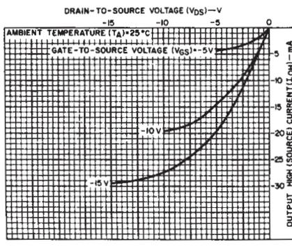
Fig. 10 - Typical output high (source) current characteristics.
