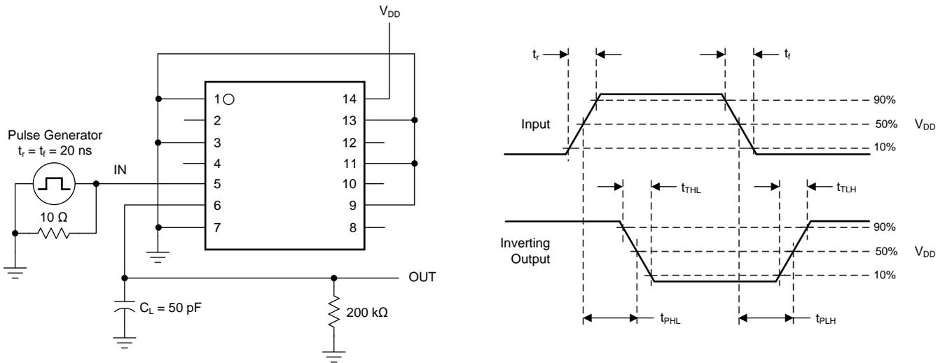
Figure 14. Dynamic Electrical Characteristics Test Circuit and Waveform
