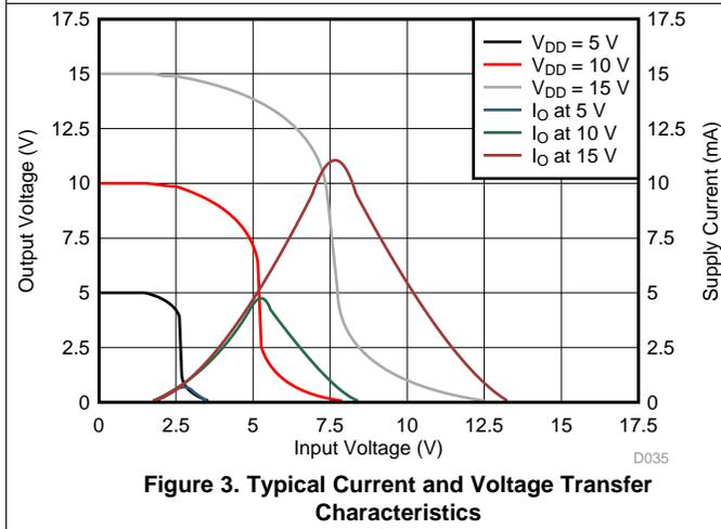
Figure 3. Typical Current and Voltage Transfer Characteristics
