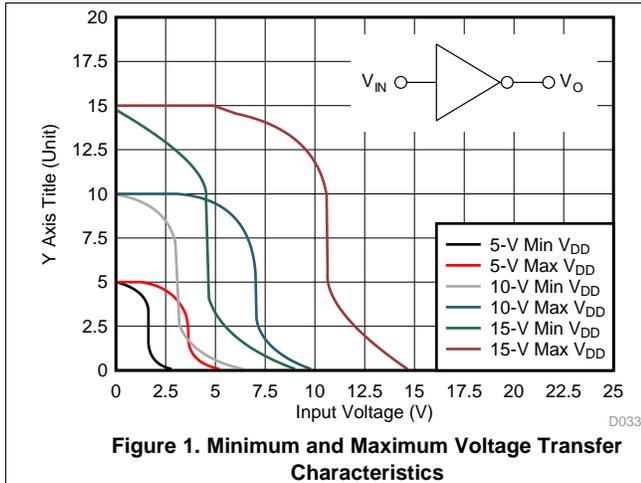
Figure 1. Minimum and Maximum Voltage Transfer Characteristics
