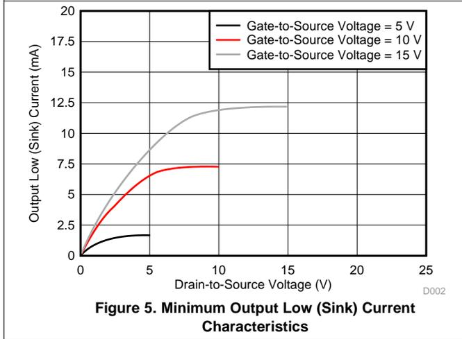
Figure 5. Minimum Output Low (Sink) Current Characteristics
