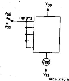
Fig. 15 - Quiescent device current test circuit.
