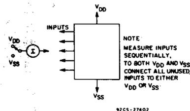
Fig. 17 - Input current test circuit.
