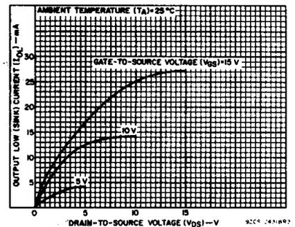
Fig. 6 - Typical output low (sink) current characteristics.
