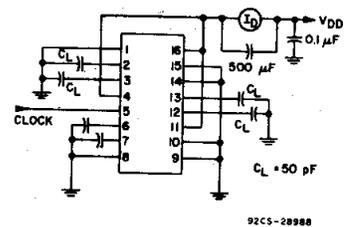
Fig. 14 - Dynamic power dissipation test circuit.
