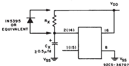
Fig. 17 - Rapid power-down protection circuit.
