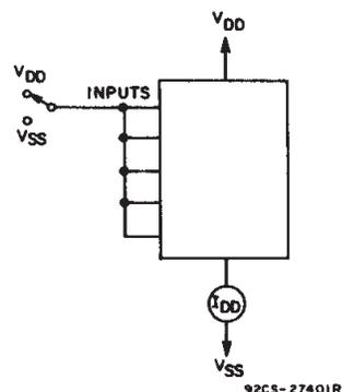
Fig. 16 - Quiescent device current test circuit.
