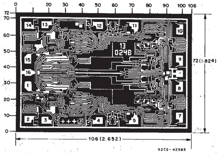
Dimensions in parentheses are in millimeters and are derived from the basic inch dimensions as indicated. Grid graduations are in mils ( $10^{-3}$  inch).
