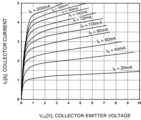
Figure 1. Static Characteristic
