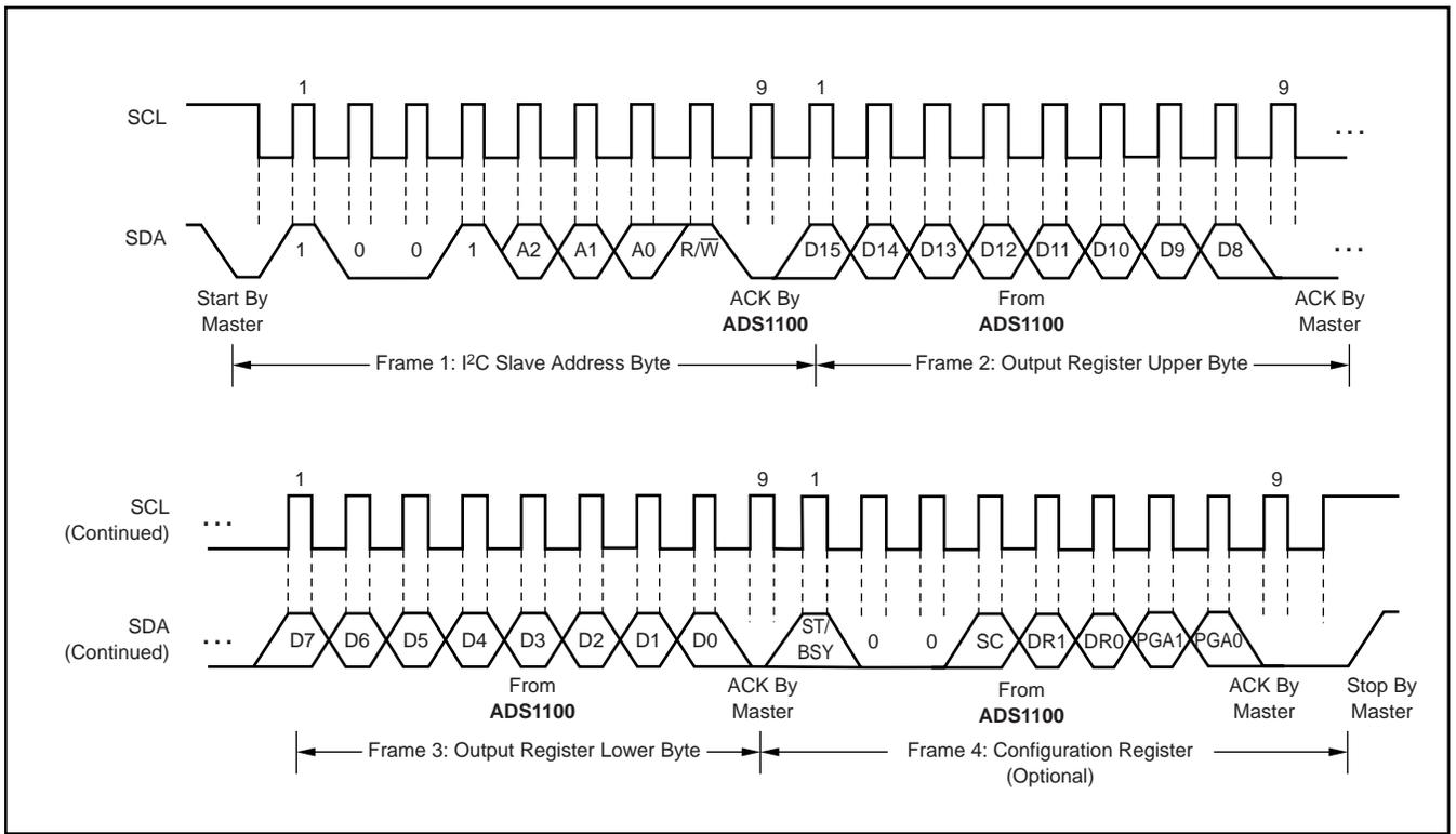
FIGURE 2. Timing Diagram for Reading From the ADS1100.
