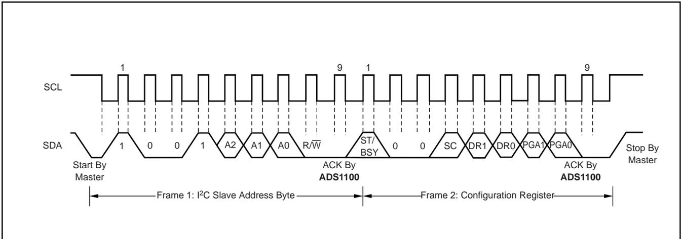
FIGURE 3. Timing Diagram for Writing to the ADS1100.
