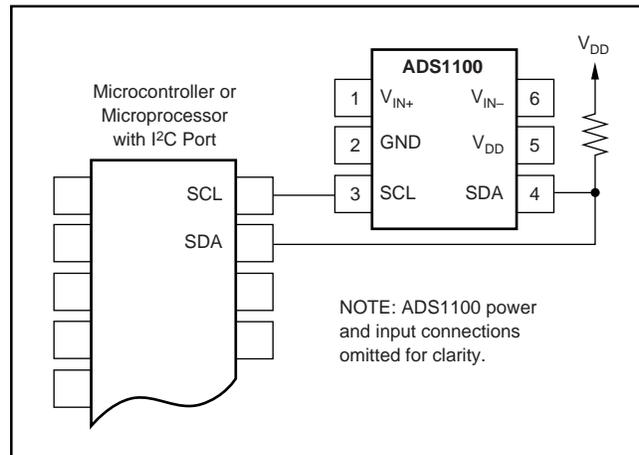
FIGURE 6. Using GPIO with a Single ADS1100.
