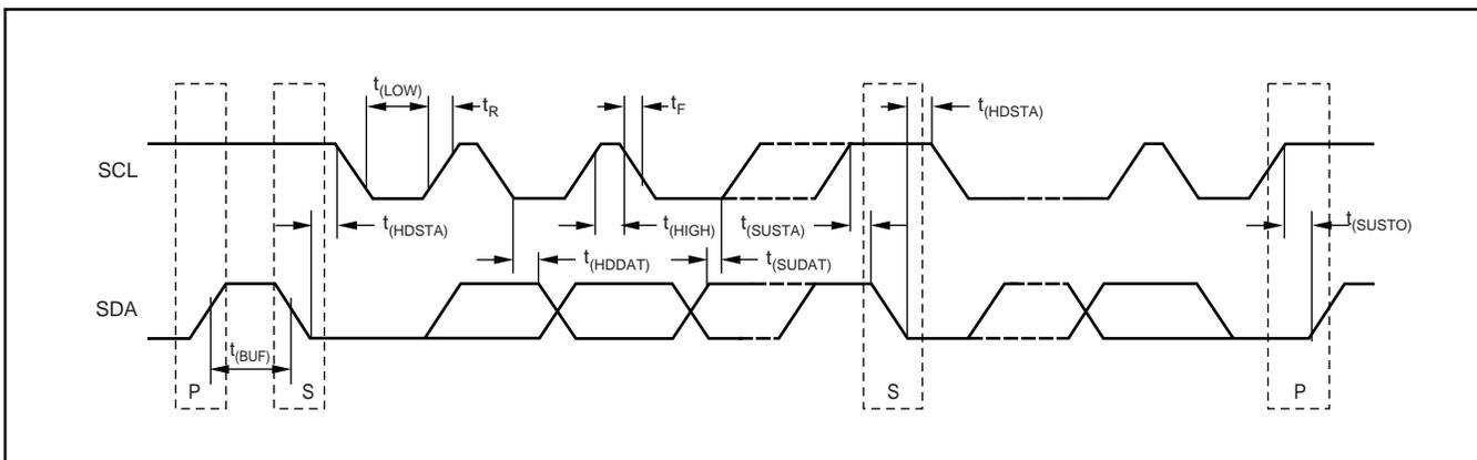
FIGURE 1. I<sup>2</sup>C Timing Diagram.
