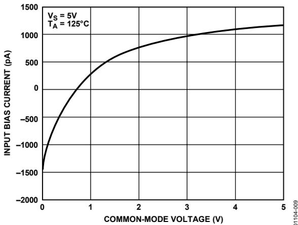
Figure 9. Input Bias Current vs. Common-Mode Voltage
