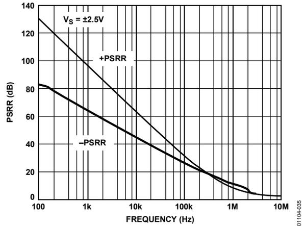
Figure 35. PSRR vs. Frequency at  $\pm 2.5V$
