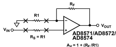
$R_S$  SHOULD BE PLACED IN CLOSE PROXIMITY AND ALIGNMENT TO  $R_1$  TO BALANCE SEEBECK VOLTAGES
