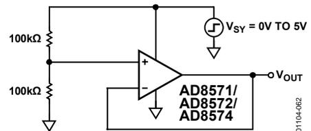
Figure 62. AD857x Test Circuit for Turn-On Time
