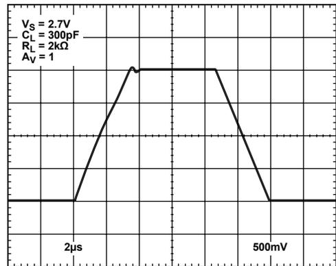
Figure 23. Large Signal Transient Response at 2.7 V
