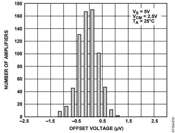
Figure 10. Input Offset Voltage Distribution at 5 V
