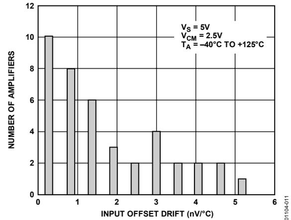
Figure 11. Input Offset Voltage Drift Distribution at 5 V
