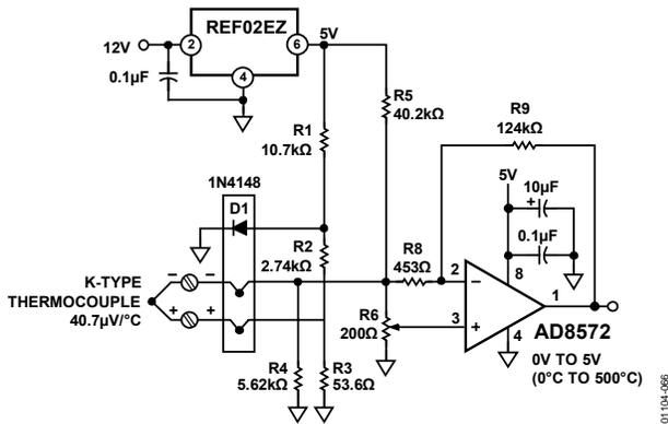
Figure 66. Precision K-Type Thermocouple Amplifier with Cold-Junction Compensation
