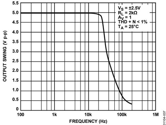
Figure 37. Maximum Output Swing vs. Frequency at 5 V
