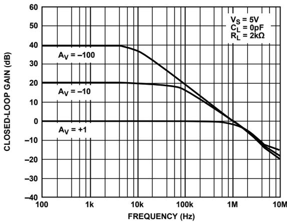
Figure 20. Closed-Loop Gain vs. Frequency at 5 V
