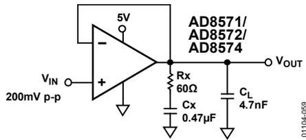
Figure 59. Snubber Network Configuration for Driving Capacitive Loads
