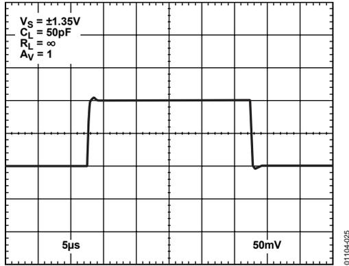
Figure 25. Small Signal Transient Response at 2.7 V
