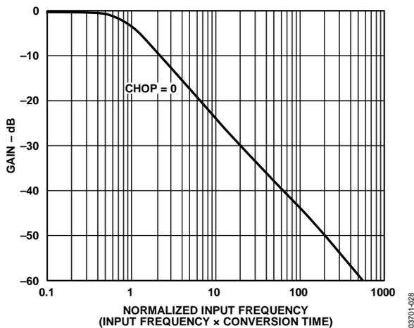
Figure 28. Typical ADC Frequency Response, Chopping Disabled
