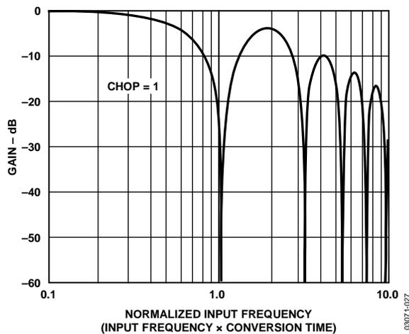
Figure 27. Typical ADC Frequency Response, Chopping Enabled
