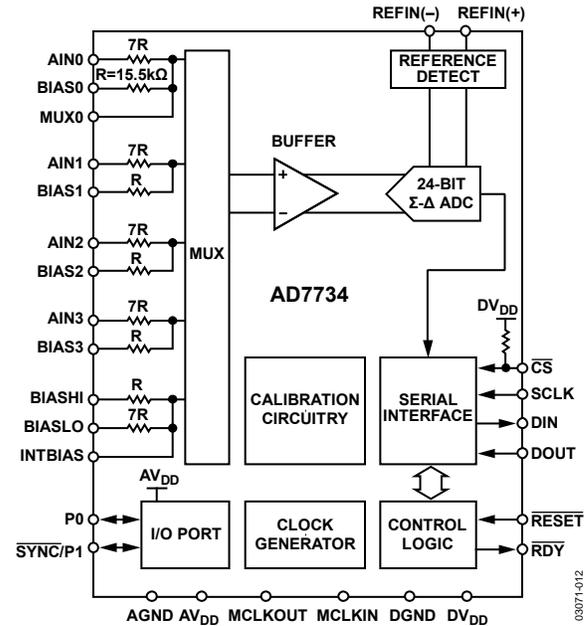
Figure 12. Block Diagram
