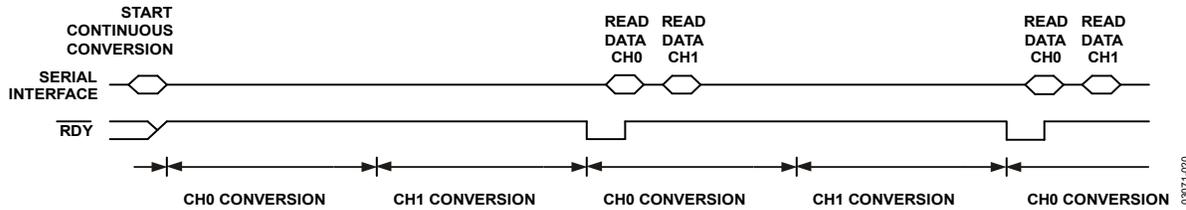
Figure 20. Continuous Conversion, CH0 and CH1, RDYFN = 1
