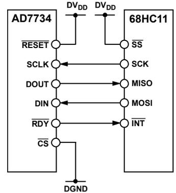
Figure 13. AD7734 to Host Device Interface, SPI
