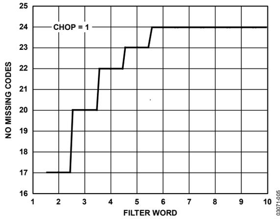
Figure 5. No Missing Codes Performance, Chopping Enabled
