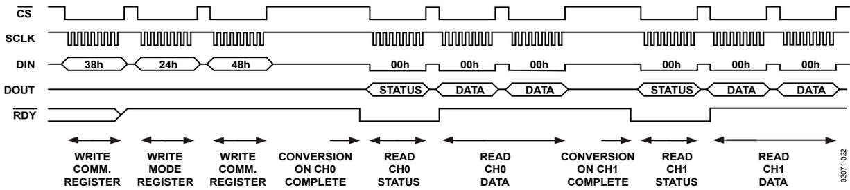
Figure 22. Continuous Conversion, CH0 and CH1, Continuous Read
