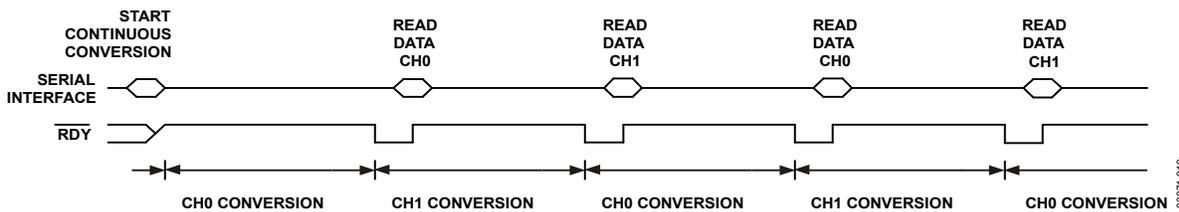
Figure 19. Continuous Conversion, CH0 and CH1, RDYFN = 0
