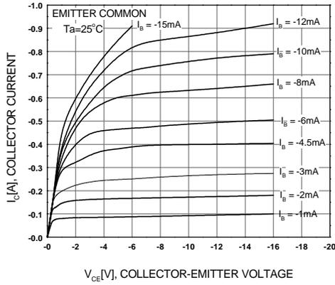
Figure 1. Static Characteristic
