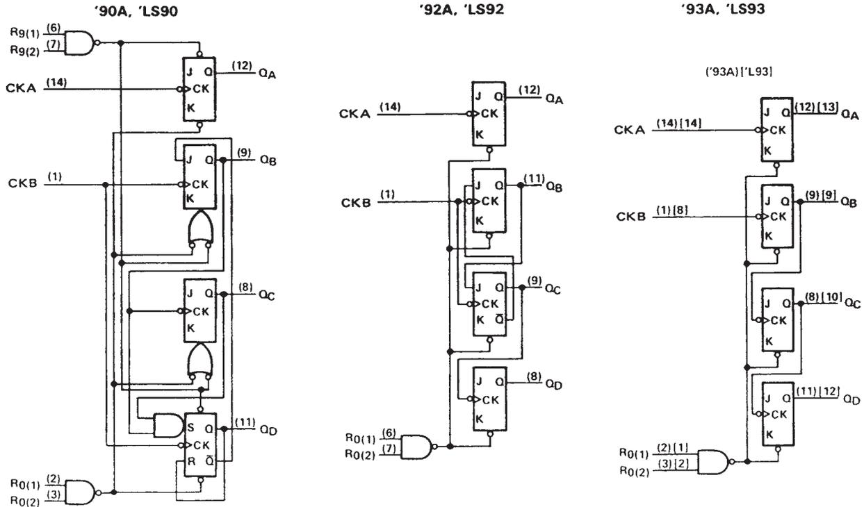
The J and K inputs shown without connection are for reference only and are functionally at a high level. Pin numbers shown in ( ) are for the 'LS93 and '93A and pin numbers shown in [ ] are for the 54L93.
