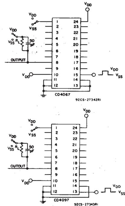
Fig. 12—Turn-on and turn-off propagation delay—
